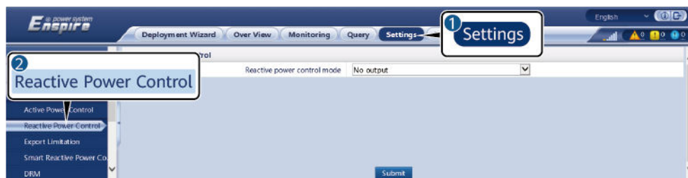
Figure 6-47 Reactive power control
